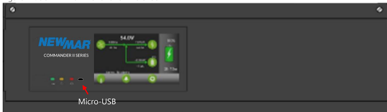
Figure 17: 3U EM4x-01 Front Panel micro-USB
