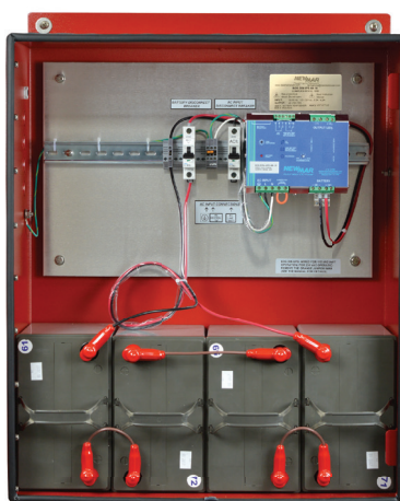
Enclosure A 12, 24, & 48V DC, 18 - 100AH
