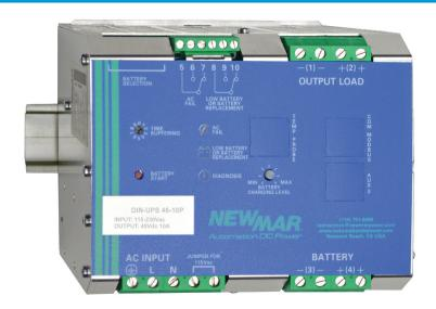
DIN-UPS "P" models can be paralleled for 1+1=2 parallel to obtain double the current of a single non-"P" model. By connecting a standard UTP Rj45 patch cable into each DIN UPS' Modbus jack on the front panel, the two "P" models will create a master and slave combination. This results in a single battery input and a single output. The master unit will display diagnostics/status for the system.
