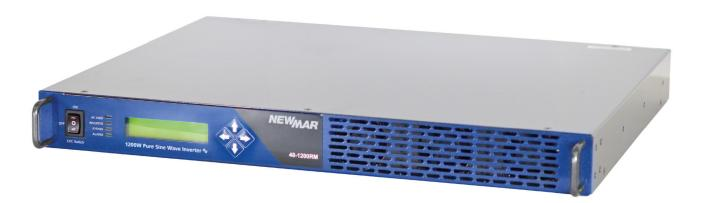
The 1U, 1200 watt, power inverter series provides seamless back-up power for AC powered communications equipment from the site's 24 or 48V DC battery system. A fast-acting transfer switch ensures voice and data transmissions remain uninterrupted in the event of a power grid failure or if the site utility power is disconnected for maintenance and upgrade purposes. Built in a compact 1U case for 19" rack installations.
