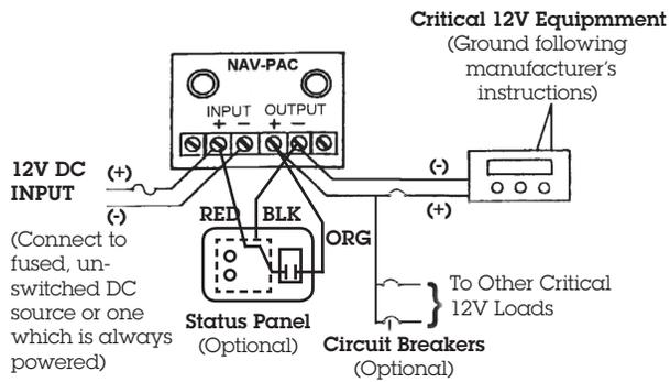
3) Optional Remote Panel: Mount in a conspicuous location where the loss of power indication will be noticed. The NAV-PAC will function normally without the remote panel or with the remote panel switch off. Connect the wiring as follows, see diagram. P/N 773-5037-0
