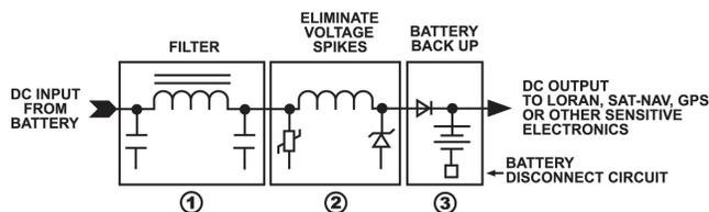
The NAV-PAC is wired in series with the DC power to sensitive electronics and:
