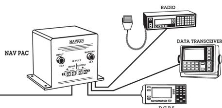
**1) Voltage Spike Protection:** Engine cranking, pump and motor operation send voltage "spikes" through a mobile electrical system that often "bulldoze" their way through the electronic circuitry. NAV-PAC eliminates this ruinous condition.
