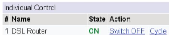
Use the keypad for local control: Select a relay using the arrow keys, then press on, off, or cycle. Press ON or OFF for 5 seconds to lock or unlock a relay. Locking prevents web access.
