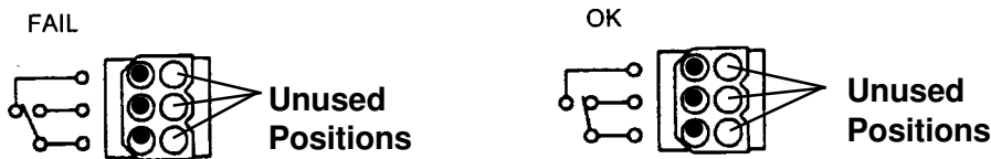
FIGURE 6: “FAIL” AND “OK” RELAY CONTACT POSITIONS
