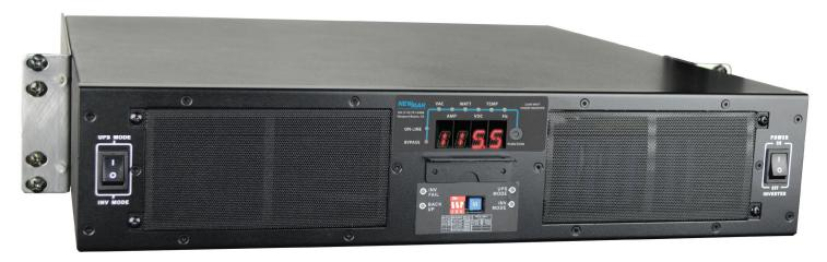
This power inverter provides seamless back-up power for AC powered communications equipment from the site's 48V DC battery system. A fast-acting transfer switch ensures voice and data transmissions remain uninterrupted in the event of a power grid failure or if the site utility power is disconnected for maintenance and upgrade purposes. Built in a 2RU case for 19" rack installations.
