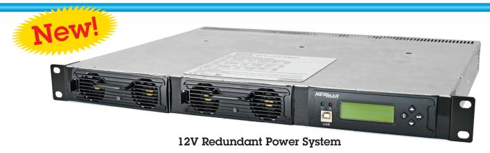
The Scout is a compact, high power density 12 volt rackmount power system that brings telecom power technology to 12 volt base station radio applications to power transmitters and maintain back-up batteries. Its dual 100 amp hot swap rectifiers configured in N+1 redundancy provides fault tolerant reliability. Remote monitoring capability provides system administrators with operating status.
