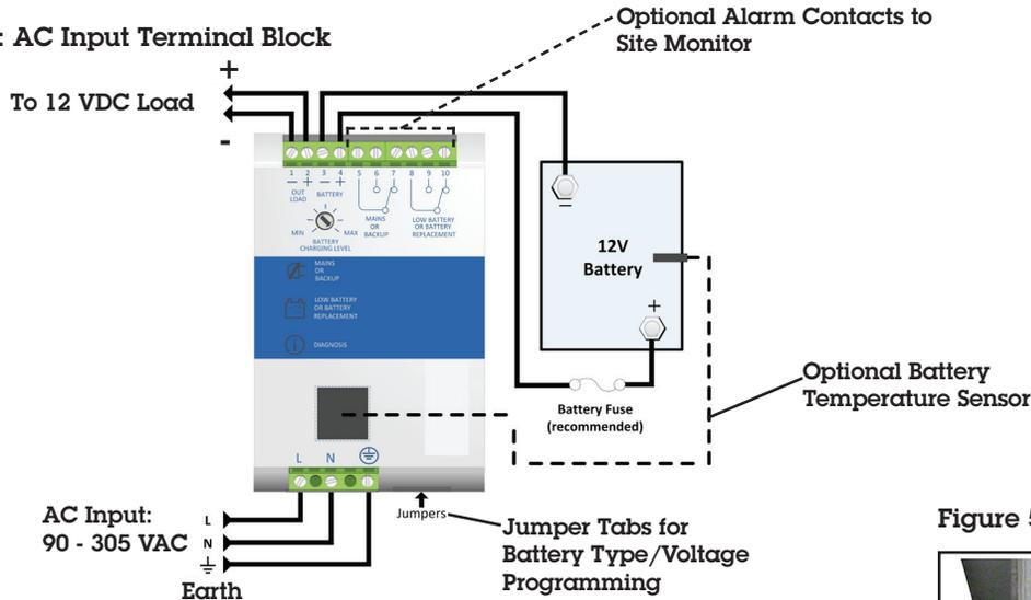
Figure 5: AC Input Terminal Block
