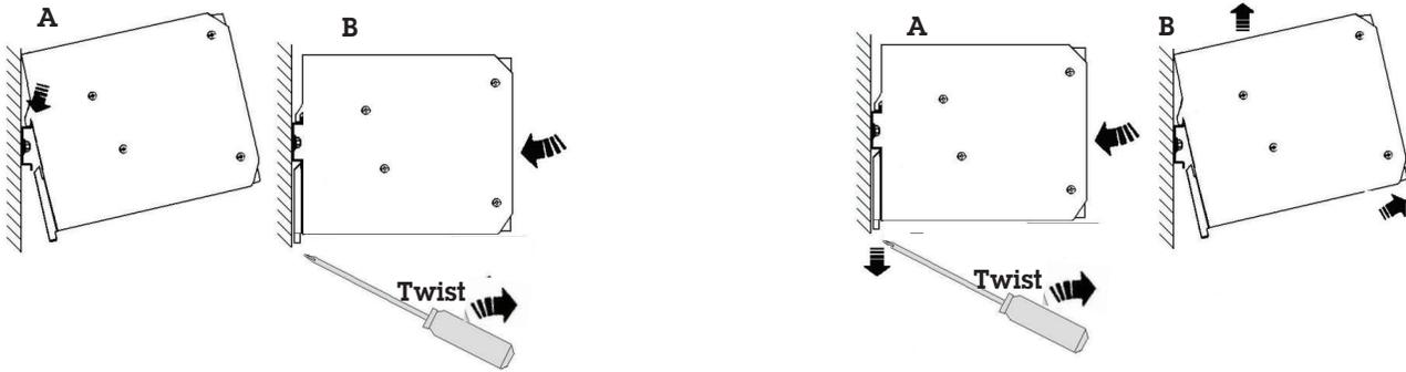
Insert flat head screwdriver in slot of bottom tab and twist to extend bracket
